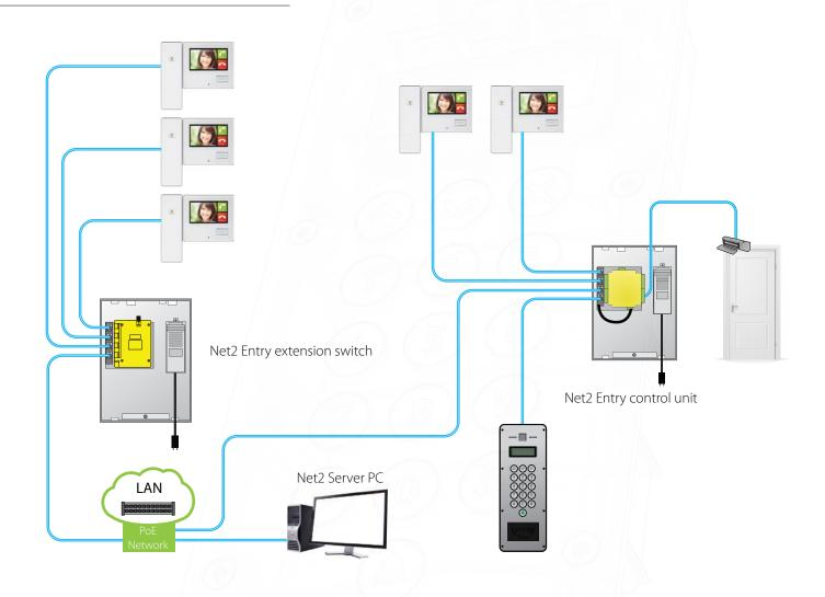
The Net2 Entry control unit has four PoE ports and one standard network port. The PoE ports can be used to power panels or monitors. All five network ports can be used for data to expand the network.
