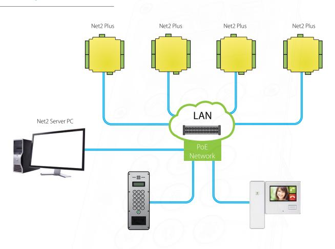
The Net2 Entry system can be fully integrated into a Net2 Access control system by simply adding panels and monitors to the existing Net2 network.
