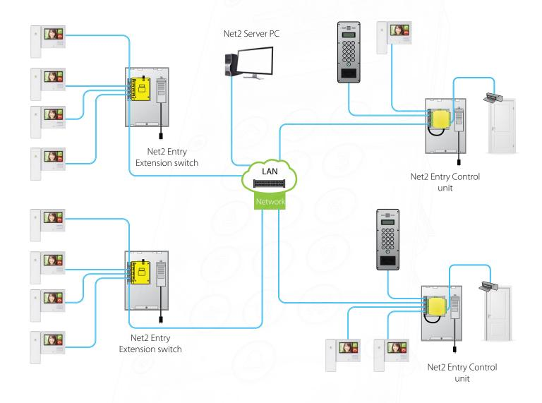
Very large systems can be configured using multiple panels and monitors.
