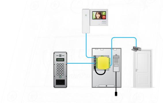
Net2 Entry can be installed as a standalone system using one control unit, one entry panel and one monitor.
